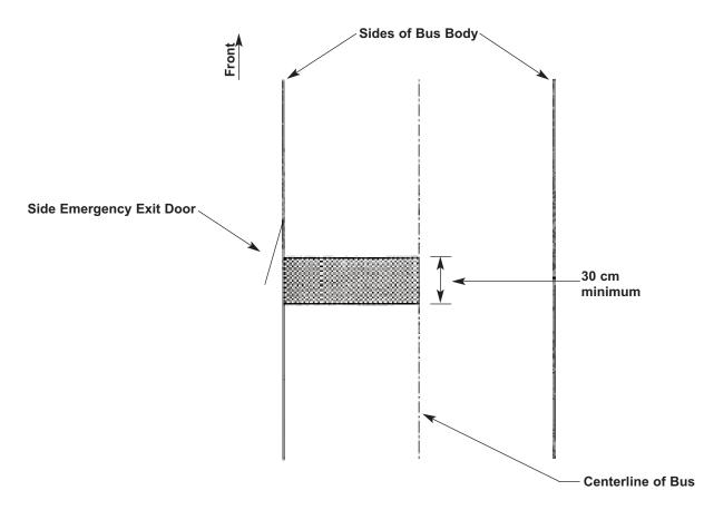
Minimum Side Emergency Exit Clearance Specifications (Plan View)
