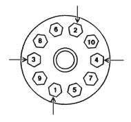
3. Torque all wheel nuts to 450-525 ft/lbs. (608-7098 Nm).
