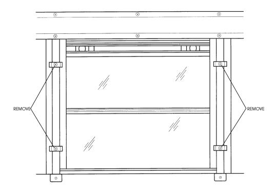
The sash is installed in the window opening and is securely anchored on both sides to the one piece bow frames with four (4) clips, two (2) on either side of the window.
