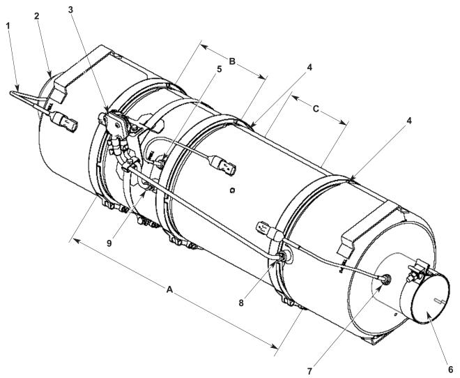
FIGURE 2- AFTERTREATMENT DEVICE (TYPICAL)
