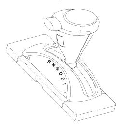
To put the transmission into gear, move the selector lever from Neutral to the desired drive position.
