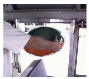
Ellipsoid gauge passing above seat back
