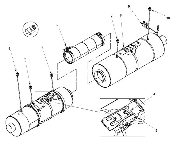
FIGURE 1 - CUMMINS ATD SENSOR LOCATIONS
