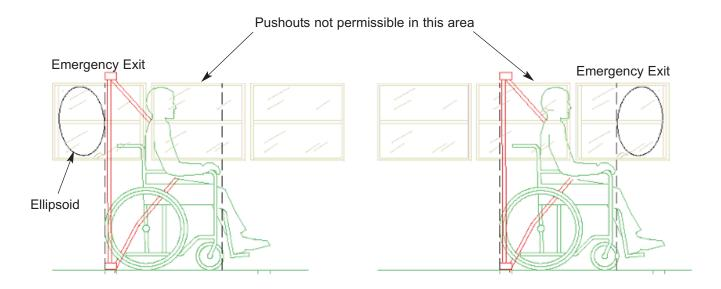
10. Removable barriers and seats should allow for a 12" clear aisle to emergency exit doors without exceeding maximum seat spacing.
