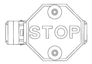
Stop arm/crossing arm assemblies are purchased as a kit, with many different kits available with blades to meet all state requirements. The assembly is attached to the outside of the outside of the body or bumper with sheet metal screws. This assembly requires occasional cleaning and lubrication of moving parts.
