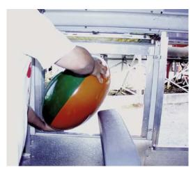
Ellipsoid gauge passing in behind of seat back
