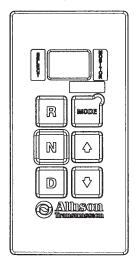
The pushbutton shift selector has R, N, D, Up Arrow, **Down Arrow**, **Mode Button**, and a digital display.
