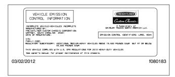
Fig. 1.8, Vehicle Emission Control Information Label
