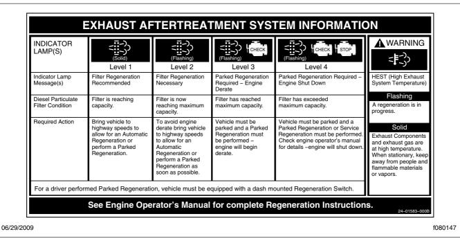
Fig. 8.1, Exhaust-Aftertreatment Warnings Reference Label
