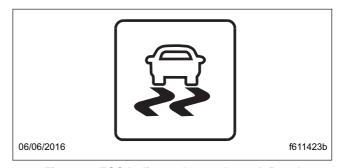
Fig. 10.4, ESC Indicator Lamp, Ametek Panel
