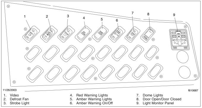
Fig. 5.9, Driver Switch Panel (typical)
