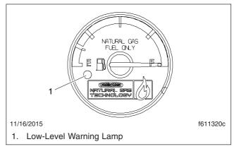
Fig. 18.9, Fuel Level Gauge
