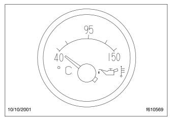
Fig. 4.19, Engine Oil Temperature Gauge
