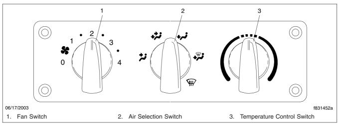
Fig. 5.25, Climate Control Panel Without Air Conditioning
