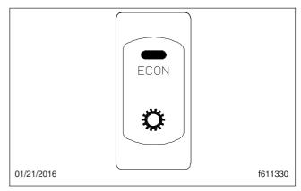
Fig. 5.20, Transmission Mode Switch
