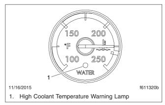
Fig. 18.11, Coolant Temperature Gauge
