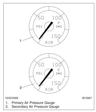
Fig. 4.14, Air Pressure Gauges
