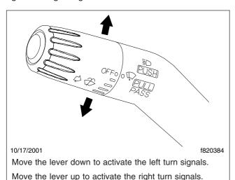
Fig. 5.6, Turn Signal Controls
