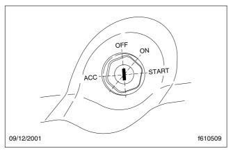
Fig. 5.1, Ignition Switch Positions
