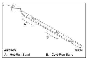
Fig. 12.4, Automatic Transmission Dipstick Markings
