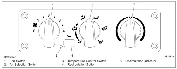
Fig. 5.26, Climate Control Panel With Air Conditioning
