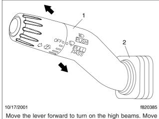
Move the lever forward to turn on the high beams. Move the lever back to its original position to turn them off.
