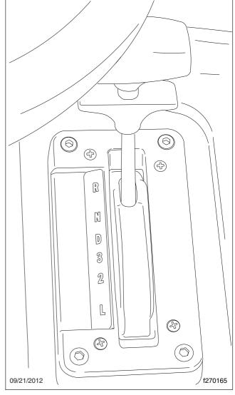
Fig. 9.1, T-Handle Shifter (standard)
