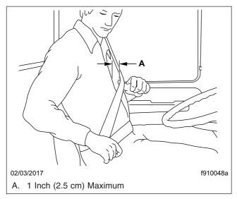
Fig. 3.15, Adjusting Shoulder Harness Clearance
