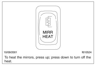
Fig. 3.2, Mirror Heat Switch
