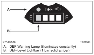
Fig. 8.5, DEF Level Low-Initial Warning
