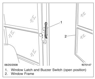
Fig. 2.12, Vertical Push-Out Window (open position)
