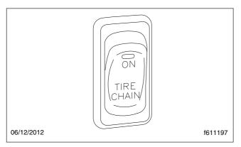
Fig. 5.12, Automatic Tire Chain Switch
