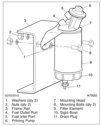
Fig. 12.5, Alliance Fuel/Water Separator Assembly and Installation
