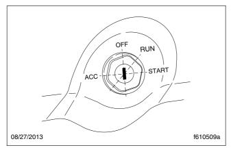
Fig. 17.2, Ignition Switch Positions
