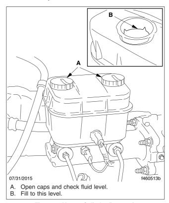
Fig. 10.2, Master Cylinder Reservoir
