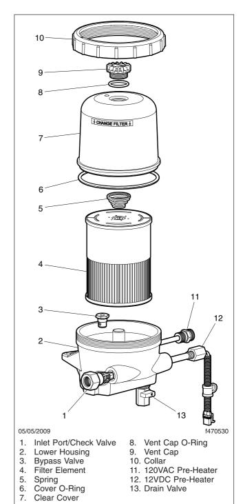
Fig. 12.6, DAVCO Fuel/Water Separator (Fuel Pro 482 shown)
