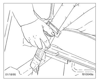
Fig. 3.17, Releasing the Three-Point Seat Belt
