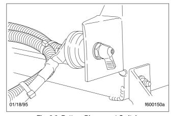
Fig. 2.6, Battery Disconnect Switch
