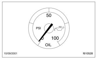
Fig. 4.11, Engine Oil Pressure Gauge
