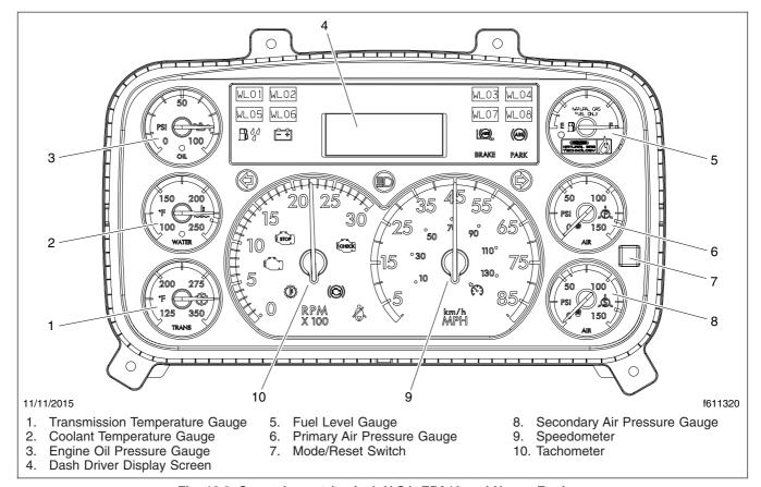
Fig. 18.3, Gauge Layout (typical, U.S.), EPA10 and Newer Engines
