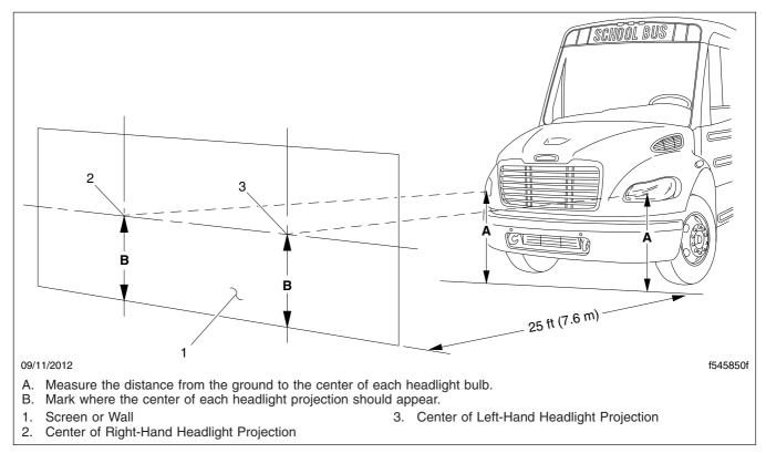
Fig. 15.2, Headlight Aiming Screen/Wall
