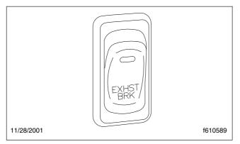
Fig. 10.5, Exhaust Brake Switch
