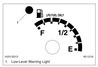
Fig. 17.21, Fuel Level Gauge
