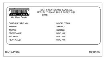
Fig. 1.2, Vehicle Data Plate
