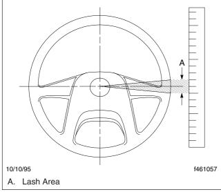
Fig. 12.14, Measuring Lash at the Steering Wheel
