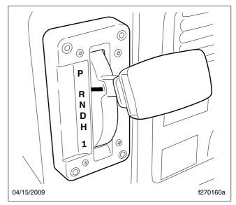
Fig. 16.4, T-Handle Shift Control (hybrid vehicle)
