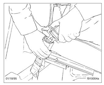
Fig. 3.14, Fastening the Three-Point Belt
