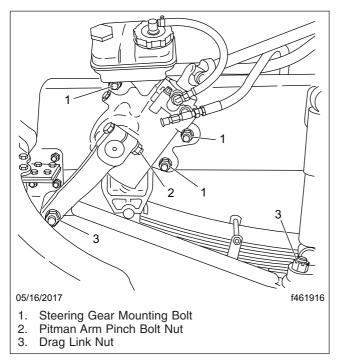
Fig. 12.12, Steering Gear Fasteners
