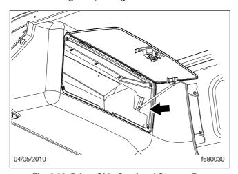
Fig. 3.20, Driver-Side Overhead Storage Box
