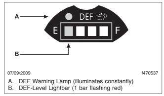
Fig. 8.6, DEF Level Low—Critical Warning
