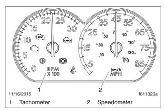
Fig. 18.8, Speedometer and Tachometer (U.S. version)
