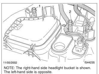
Horizontal (inboard) Adjusting Knob
