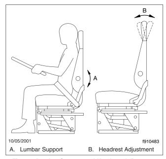
Fig. 3.5, Lumbar Support and Headrest Adjustment
