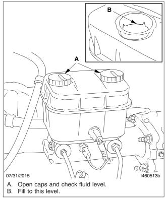
Fig. 12.13, Hydraulic Brake Reservoir
