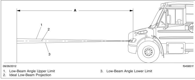
Fig. 15.3, Vertical Low-Beam Headlight Variation Limits
