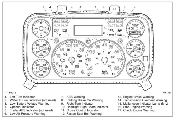
Fig. 18.5, ICU3S Warning and Indicator Lamps, EPA10 and Newer Engines
