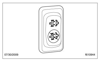
Fig. 8.3, Regen Inhibit Switch (optional when available)
