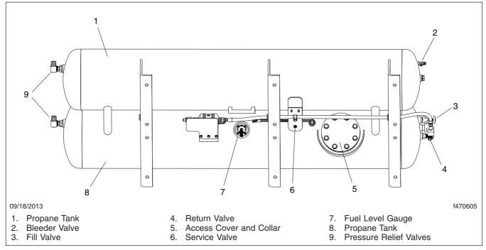
Fig. 17.4, Dual Propane Tank System
