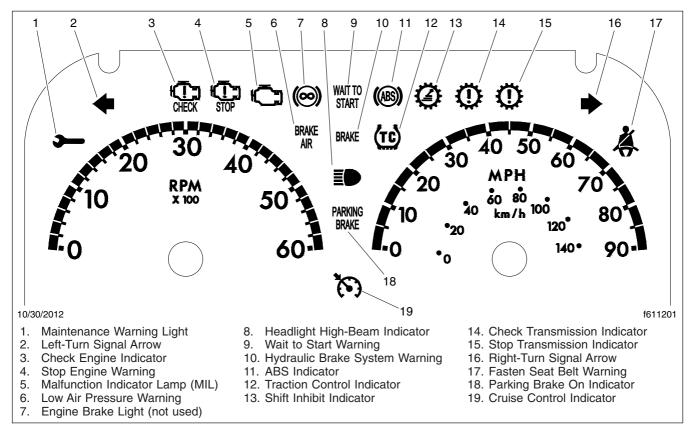
Fig. 17.19, LPG Engine Warning and Indicator Lights
