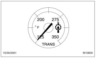
Fig. 4.21, Transmission Fluid Temperature Gauge
