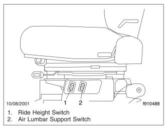
Fig. 3.13, Air Controls, Sears Seat
