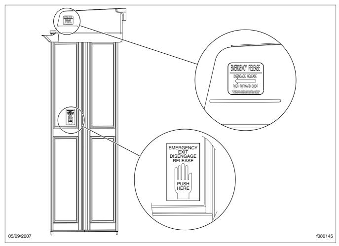
Fig. 2.10, Disengaging the Main Entry Door in an Emergency
