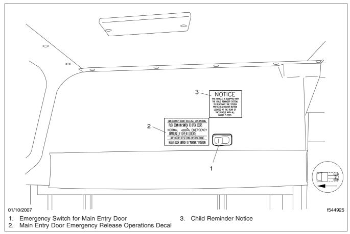
Fig. 14.6, Emergency Switch for Main Entry Door
