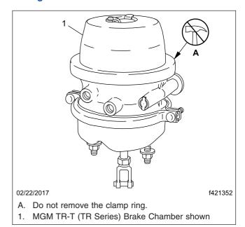
Fig. 12.8, Parking Brake Chamber Clamp
