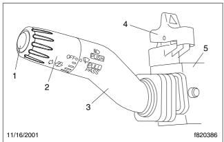
Press down on the upper part of the rocker to activate the hazard warning lights.
