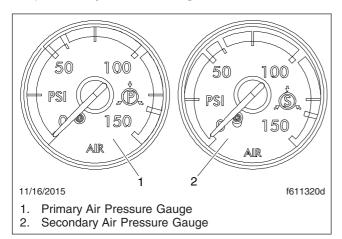
Fig. 18.10, Air Pressure Gauges
