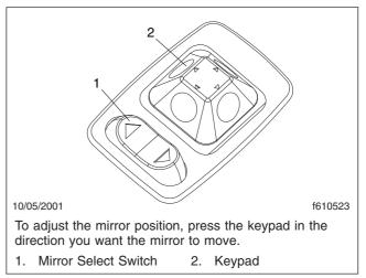
Fig. 3.3, Power Mirror Switch Pad
