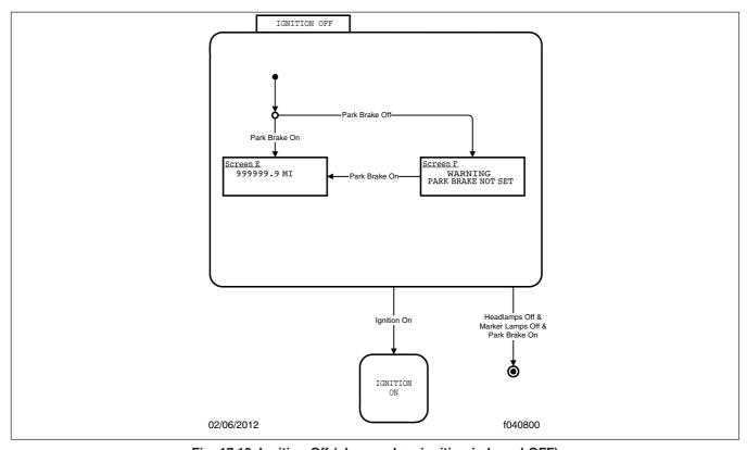
Fig. 17.18, Ignition Off (shown when ignition is keyed OFF)
