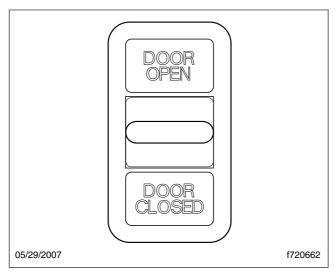
Fig. 2.3, Door Open/Door Closed Paddle Switch
