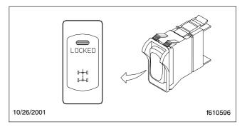
Fig. 5.21, Differential Lock Switch
