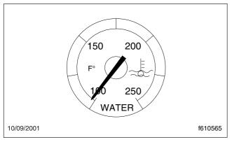
Fig. 4.12, Coolant Temperature Gauge
