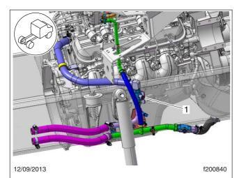
To close the valve, it must be rotated 90 degrees so that it is perpendicular to the coolant lines.
