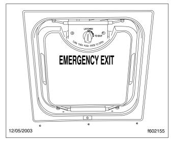
Fig. 2.8, Emergency Roof Escape Hatch
