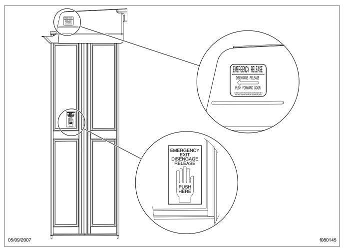
Fig. 14.7, Disengaging the Main Entry Door in an Emergency
