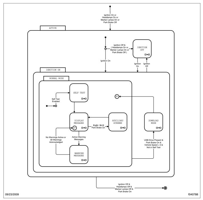
Fig. 17.10, Ignition On, Normal Mode
