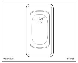
Fig. 12.7, Pretrip Light Inspection Switch
