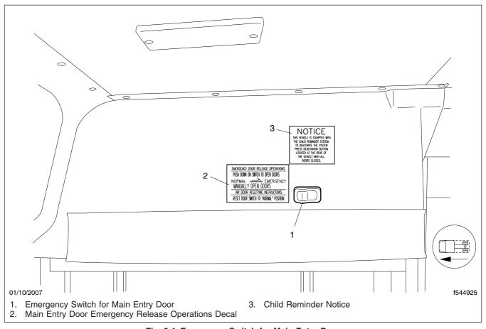
Fig. 2.4, Emergency Switch for Main Entry Door
