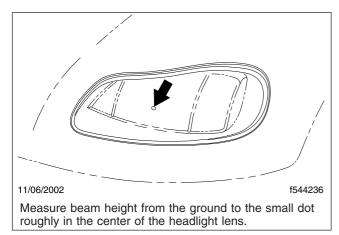
Fig. 15.1, Headlight Beam Height Adjusting Dot
