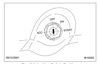
Fig. 18.2, Ignition Switch Positions
