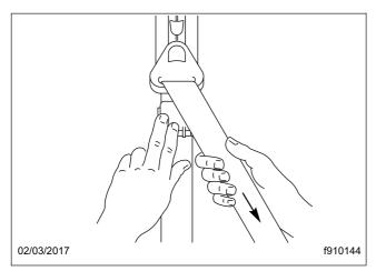
Fig. 3.16, Locking the Komfort Latch
