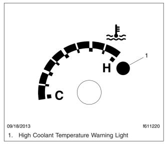
Fig. 17.23, Coolant Temperature Gauge
