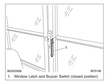
Fig. 2.11, Vertical Push-Out Window (closed position)
