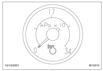
Fig. 4.22, Turbo Boost Pressure Gauge
