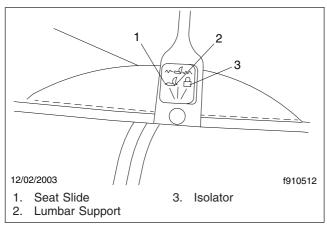
Fig. 3.4, Seat Slide and Isolator Lever
