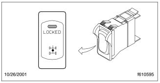
Fig. 5.22, Interaxle Lock Switch
