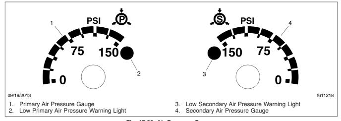
Fig. 17.22, Air Pressure Gauges
