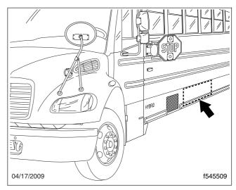
Fig. 16.3, High Voltage Cables and Power Electronics Carrier (PEC) Location
