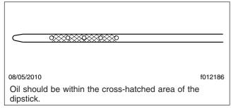
Fig. 12.3, Oil Dipstick (propane engine)
