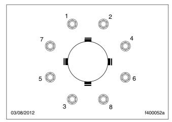
Fig. 12.11, Tightening Pattern, 8-Stud Disc Wheels
