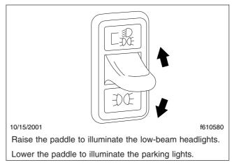
Fig. 5.2, Headlight/Parking Light Switch
