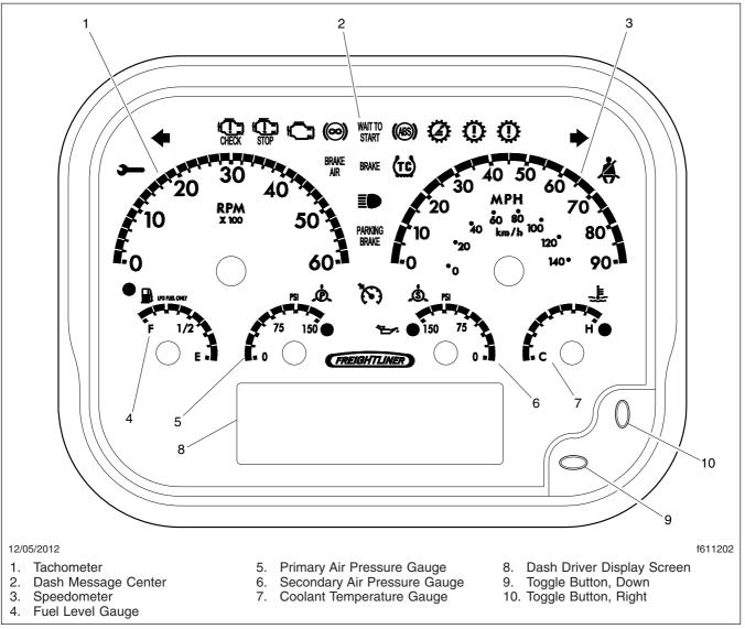
Fig. 17.5, Gauge Layout (typical, U.S.), LPG Engines
