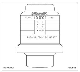
Fig. 4.15, Air Intake Restriction Indicator
