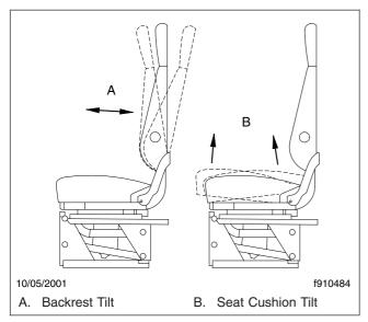
Fig. 3.6, Cushion Tilt Adjustments
