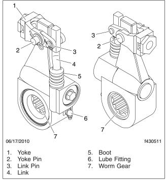
Fig. 5, Bendix Automatic Slack Adjuster
