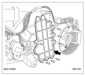
Fig. 1, HVAC Cover Removal
