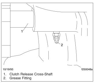
Fig. 3, Cross-Shaft Grease Fitting, Left Side
