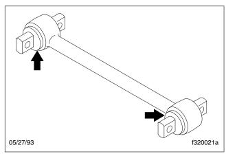
Fig. 1, Torque Arm Bushings
