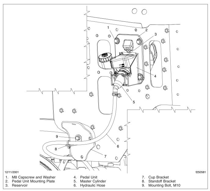
Fig. 7, Clutch Master Cylinder
