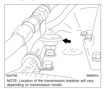
Fig. 2, Transmission Breather (Eaton Fuller shown)
