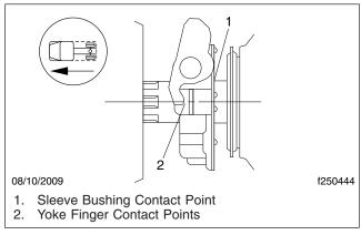
Fig. 2, Contact Points Requiring Grease
