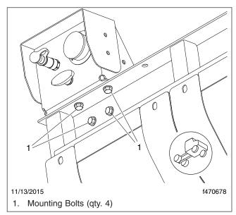
Fig. 5, Fuel Panel Mounting Bolts
