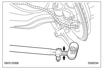
Fig. 5, Checking Tie Rod End Movement
