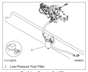
Fig. 8, Low-Pressure Fuel Filter
