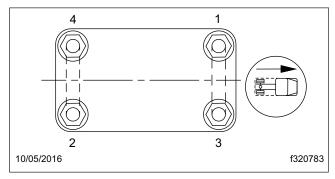
Fig. 3, Tightening Sequence for U-Bolt High Nuts
