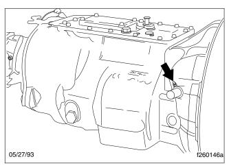
Fig. 4, Cross-Shaft Grease Fitting, Right Side
