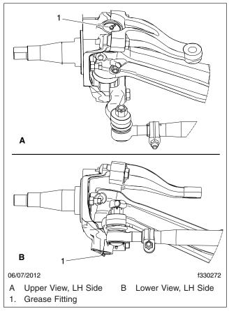
Fig. 1, Grease Fittings, Detroit Axles
