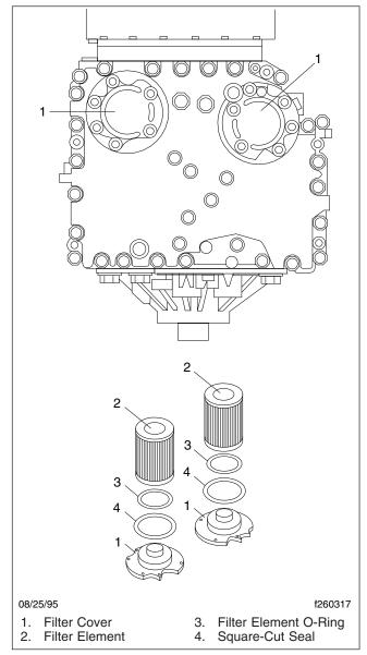
Fig. 4, Allison 3000 Series Transmission Filter Location and Components
