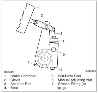
Fig. 4, Meritor Automatic Slack Adjuster
