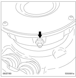
Fig. 1, Release Bearing Grease Fitting
