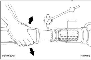
Fig. 2, Checking for Radial Looseness of the Slip Yoke Spline
