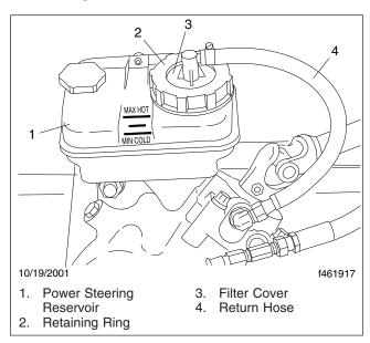
Fig. 1, Power Steering Reservoir
