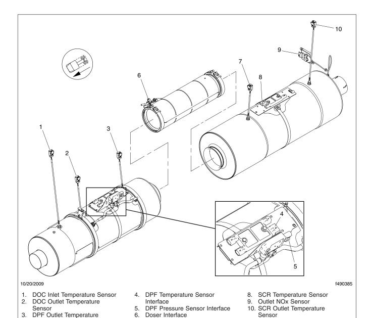
7. SCR Inlet Temperature Sensor
