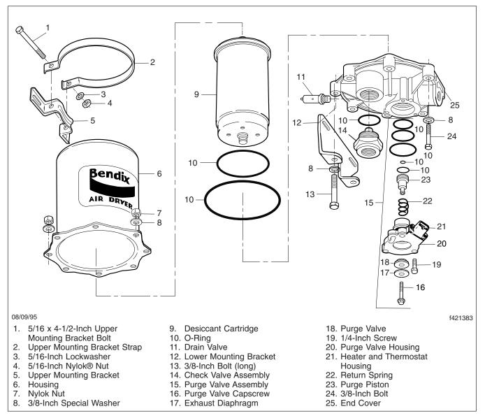
Fig. 1, AD-9 Air Dryer
