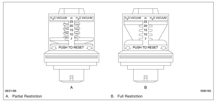
Fig. 1, Air Restriction Indicator, Diesel Engines
