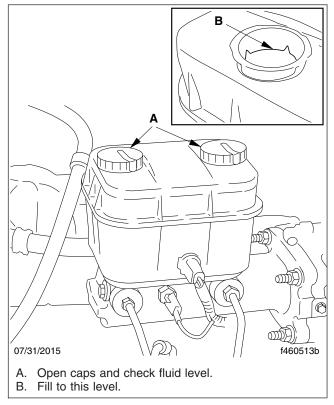
Fig. 7, Hydraulic Brake Fluid Reservoir
