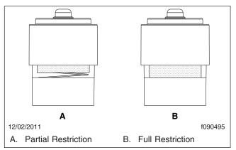
Fig. 2, Air Restriction Indicator, Propane Engines
