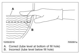
Fig. 3, Axle Lubricant Level Inspection
