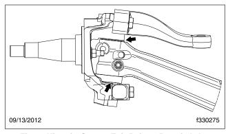
Fig. 2, Kingpin Grease Exit Points, Detroit Axles
