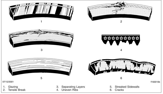
Fig. 1, Drive Belt Replacement Conditions
