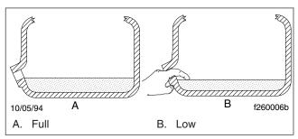
Fig. 1, Transmission Oil Level Checking
