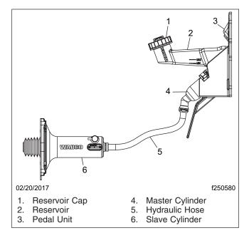
Fig. 5, Clutch Components
