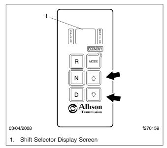
Fig. 6, Transmission Shift Selector
