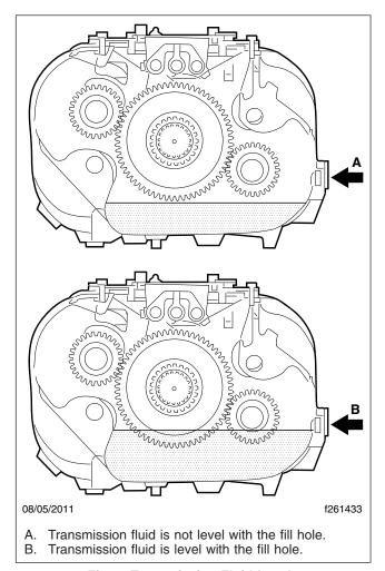
Fig. 7, Transmission Fluid Levels
