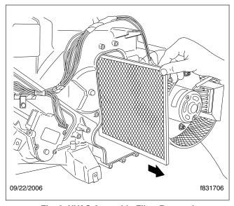
Fig. 2, HVAC Assembly Filter Removal
