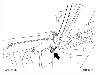
Fig. 8, Cross Shaft Grease Fitting for HEVs
