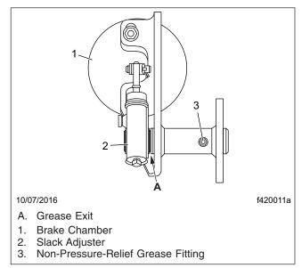
Fig. 6, Camshaft Bracket Lubricating
