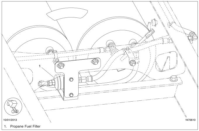
Fig. 3, Fuel Filter Location (fuel going in the tank)
