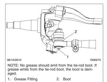
Fig. 3, Grease Fitting and Boot, Detroit Axle
