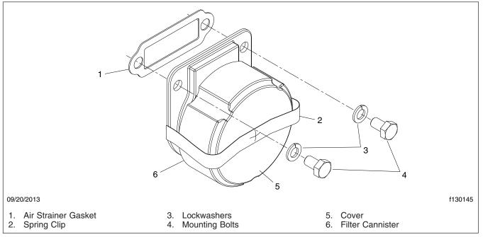
Fig. 1, Pleated Paper Filter Assembly
