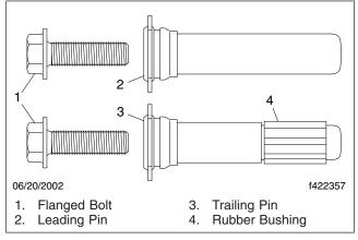
Fig. 8, ZOH-T Slide Pins and Bolts
