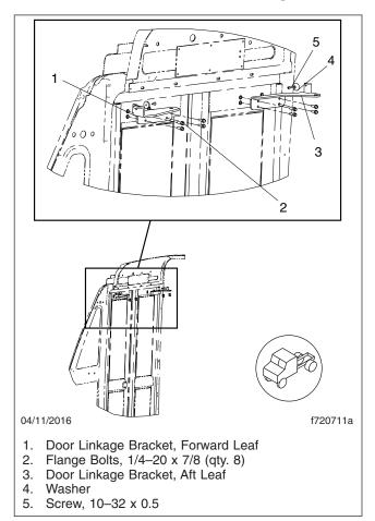
Fig. 1, Tightening the Flange Bolts
