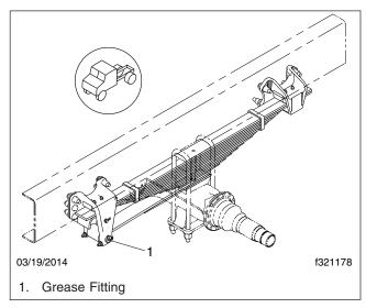
Fig. 2, Grease Fitting, Freightliner Leaf Spring Rear Suspension
