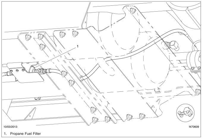
Fig. 4, Fuel Filter Location, (fuel going in the engine)
