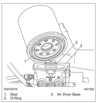
Fig. 9, Desiccant Cartridge Replacement
