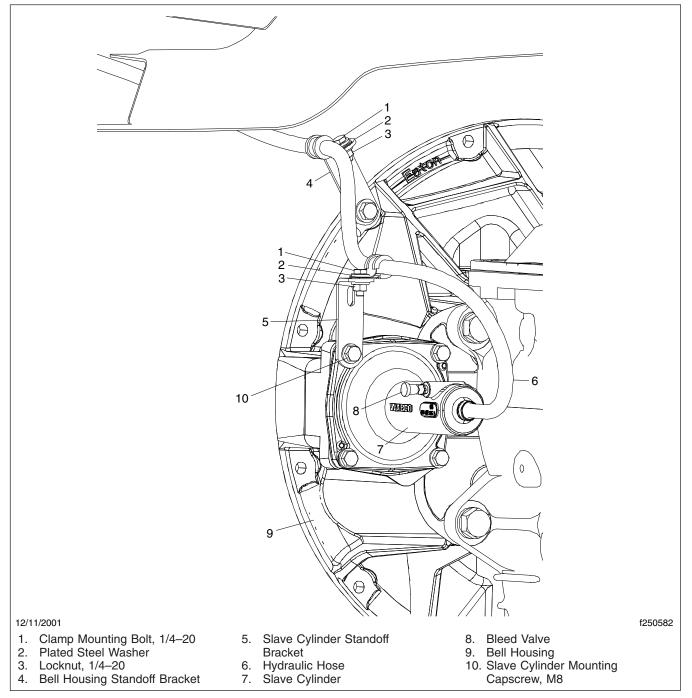
Fig. 6, Clutch Slave Cylinder
