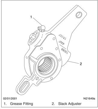
Fig. 3, Haldex Slack Adjuster Grease Fitting
