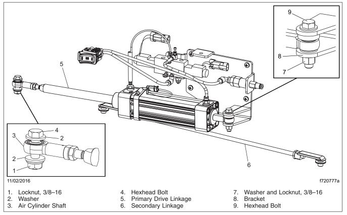
Fig. 2, Air Door Drive Linkage
