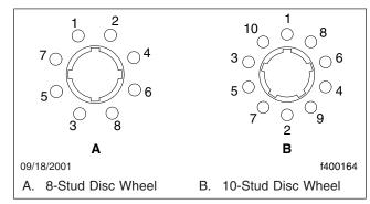
Fig. 1, Wheel Nut Tightening Sequence
