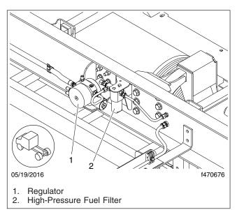
Fig. 7, High-Pressure Fuel Filter
