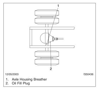
Fig. 2, Component Locations, Meritor Axles
