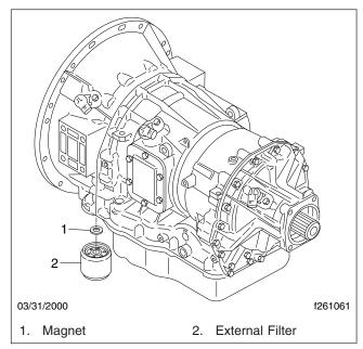
Fig. 3, 2100/2200/2500 Series Transmission External Filter
